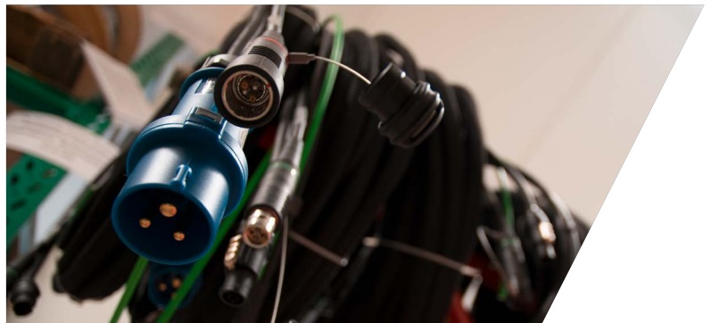
Multi Fiber Cable for the SMPTE camera signal, video signal, network, and power supply
